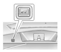
Press and release  $\leftarrow$  on the liftgate adjacent to the latch to close the liftgate.
